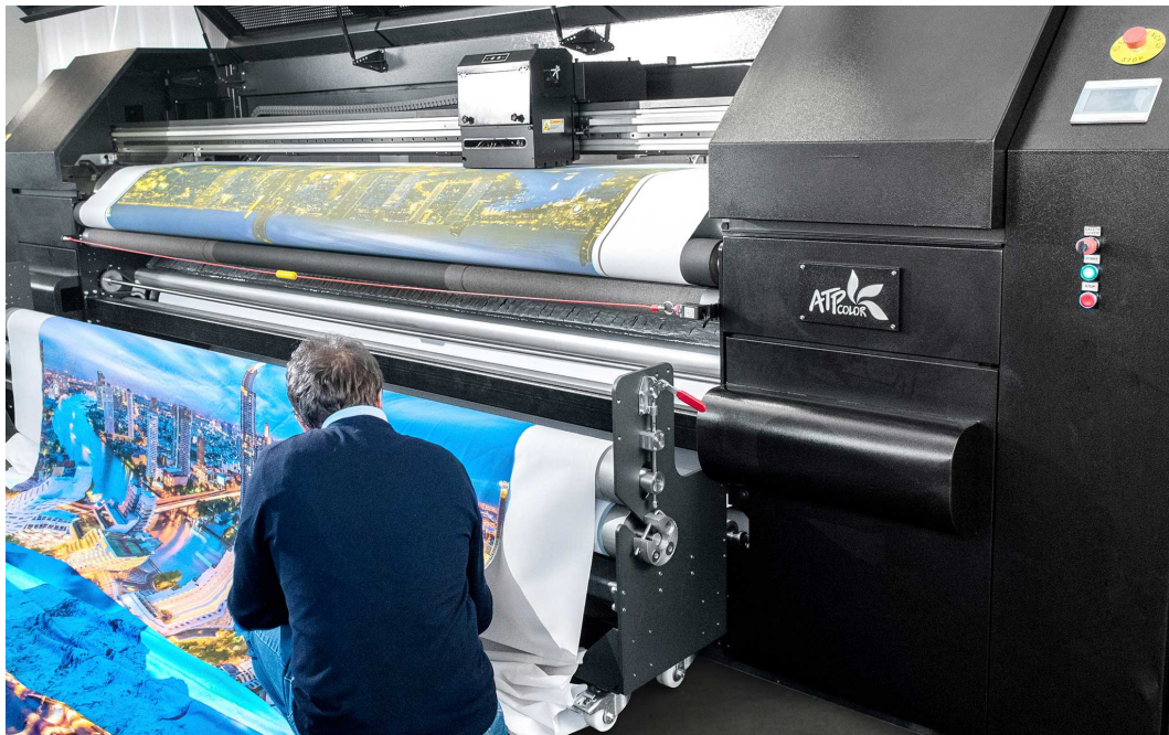
Direct-to-fabric printing and dye sublimation on ATPColor DFP56-EW.
