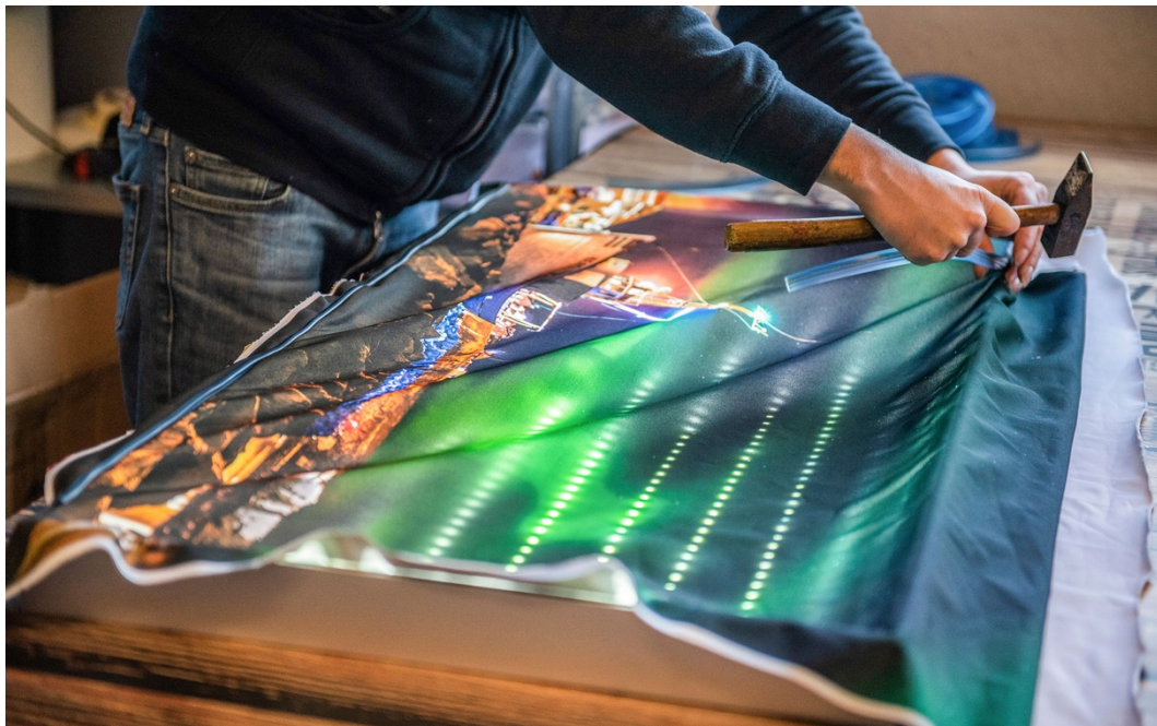
Realization of a backlit box with fabric printing.
