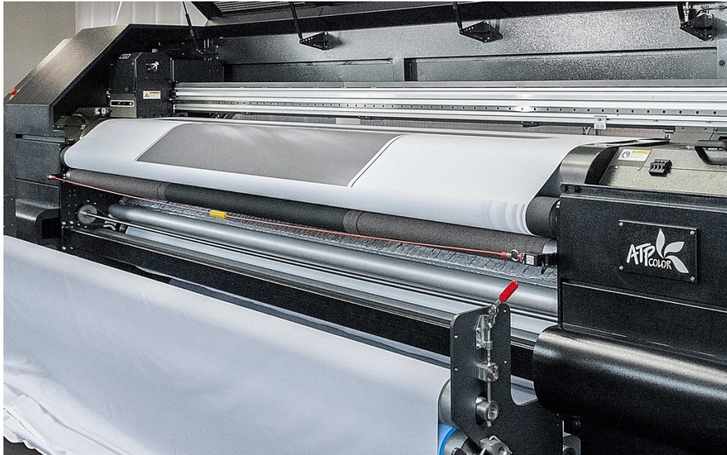
The 3.3-meter-wide ATPColor DFP-56EW sublimation printer installed by Idealgraphics in 2020.
